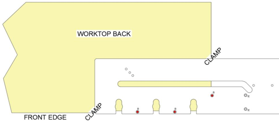
For the left hand, female bolt slots the worktop is face down as well as the jig. With pegs pushed into the holes “B”.
