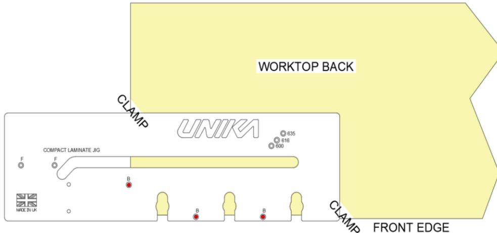
With the worktop face down and the jig face up, pegs should be pushed into the three holes marked “B”. The jig must then be placed on the reverse face of the worktop so that the two pegs between the bolt cut outs fit tightly against the female cut edge and the third peg sits tightly against the edge of the worktop. When all three pegs are in contact with the worktop the jig should be clamped in place, checking that none of them have moved out of place when tightening.
