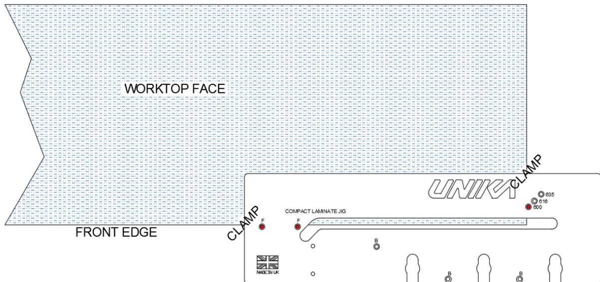
For this cut the worktop must be face up and the jig also face up. Pegs should be placed in the two holes labelled “F” and also 1 x peg to set the length of cut (in the diagram above 600 mm).
