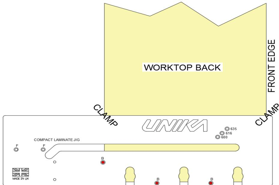
For these slots the jig is required to be face up with three pegs in the holes labelled "B" and the jig clamped in place as shown in the diagram above. Once clamped in place the routing process described on page 6 should be carried out.
