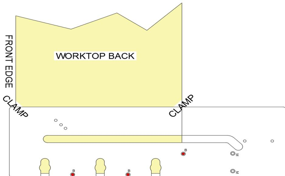
For these slots the worktop is face down as is the jig with pegs pushed into the three holes labelled “B”. With the jig on the worktop the two pegs between the bolt slots should be tight up against the male cut edge and the third peg tight up against the back edge of the worktop. Once all three pegs are in position the jig should be clamped in place and the routing process described on page 6 carried out.
