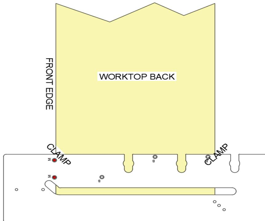
For this cut the worktop must be face down and the jig will also be face down, as shown in the diagram above.
