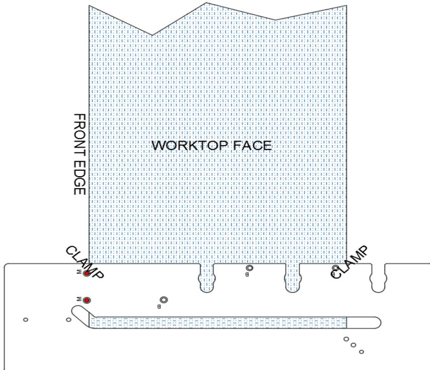
Once again the routing procedure should be followed, ensuring that the pegs remain tight to the worktop once the jig has been clamped and the router is only moved in a left to right direction with the final pass being performed as described earlier.
